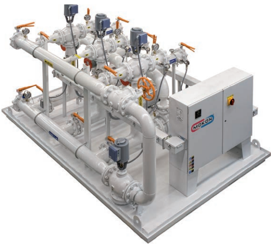
Process heating and cooling skid-mounted water temperature control system with NEMA 12 electrical components and 3 zones of control – two at 600 GPM each and third zone 400 GPM.
