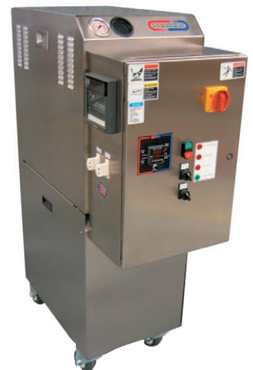
Closed-circuit temperature control system with stainless steel cabinetry including electrical enclosure and louvered panels for wash down capabilities, and 2-pen temperature chart recorder.
