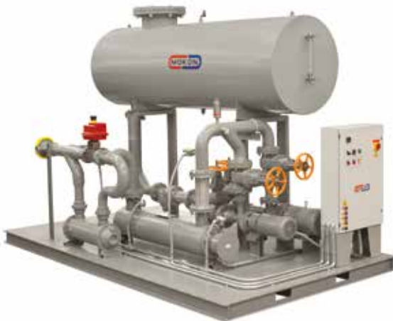
Custom oil skid-mounted temperature control system with flow regulation of five zones. NEMA 12 design with 270 GPM flow, 36 kW process heaters, and expansion tank.
