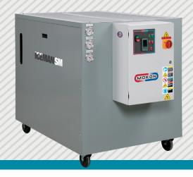
Mokon's Iceman SM Series portable chiller maximizes performance with process cooling from 20°F to 65°F (-7C to 18°C). The Iceman SM Series features a digital scroll compressor capable of providing variable capacity output from 10% to 100%.
